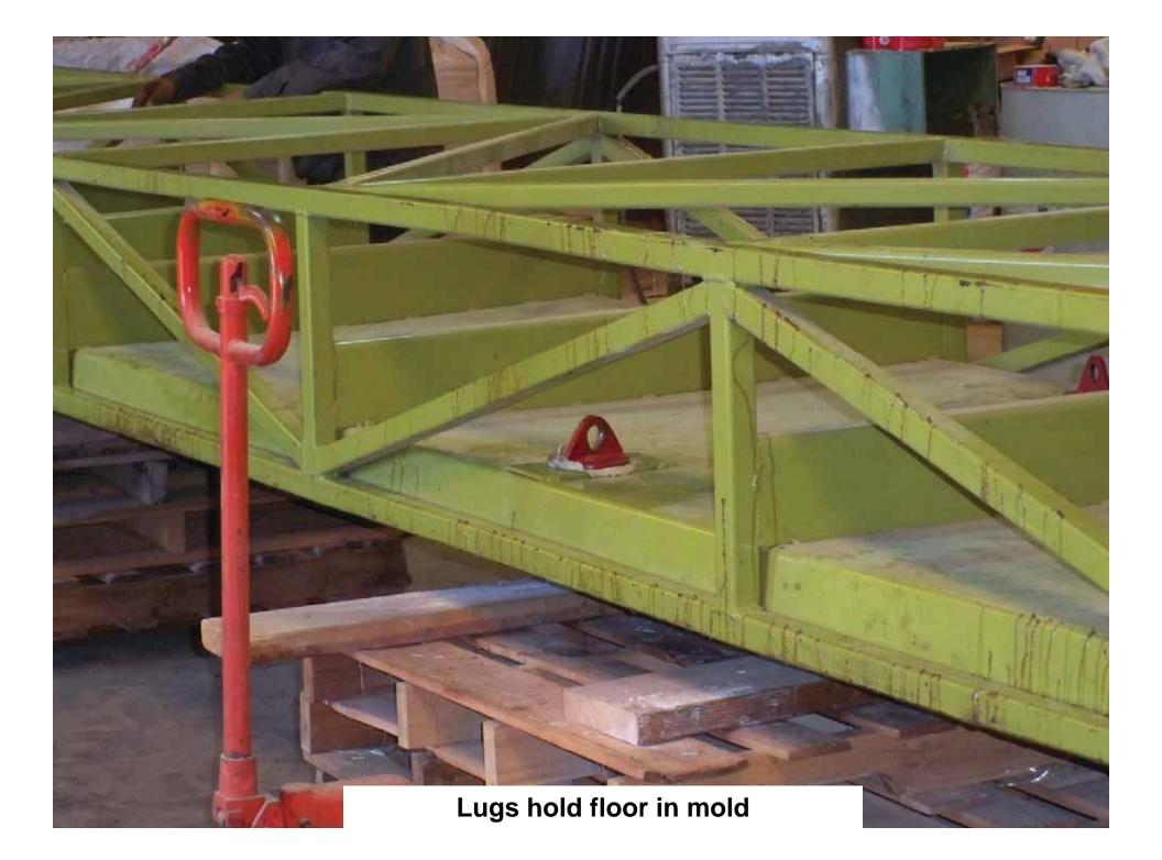
Floor is demolded and lugs re-inserted to assist in transporting floor
