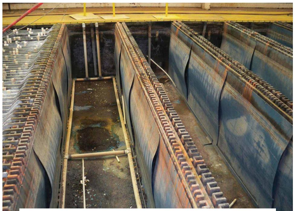
Concrete Cell with Paraliner after removal of electrodes and electrolyte
